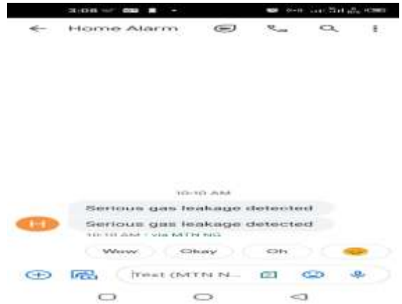
Figure 20: Display of SMS for Leakages
