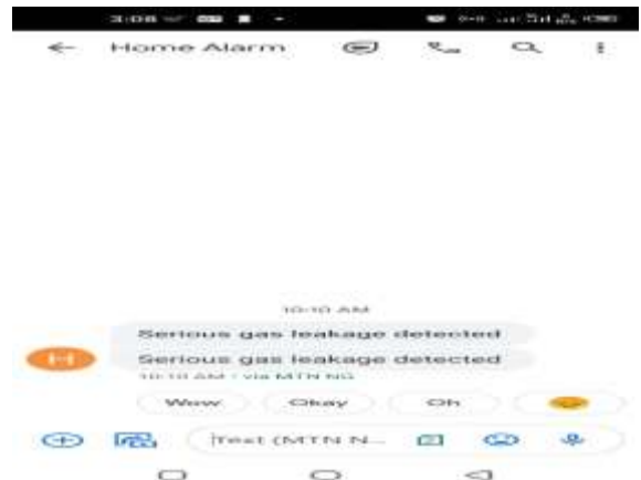
Figure 20: Display of SMS for Leakages
